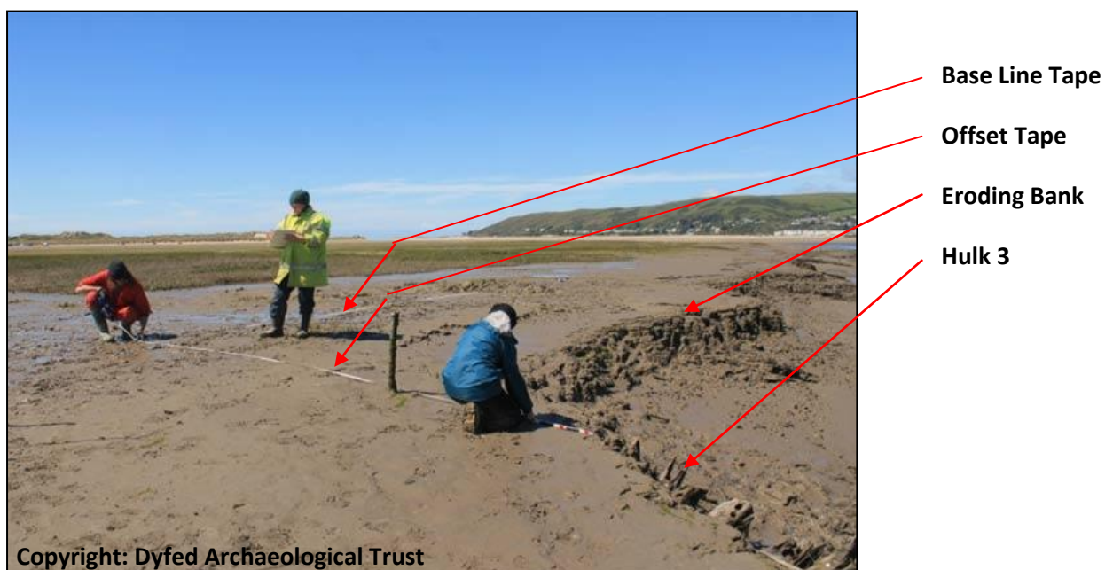
Figure 6. Carrying out an Offset Survey of the Afon Leri's eroding bank (DAT).
