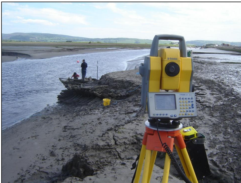
Figure 11. The total station ready for action.
