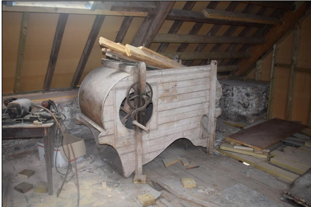
Fig. 13 Winnower and flooring on the upper floor of the granary including remnant skirting boards behind it Photo CPAT 4691-53
