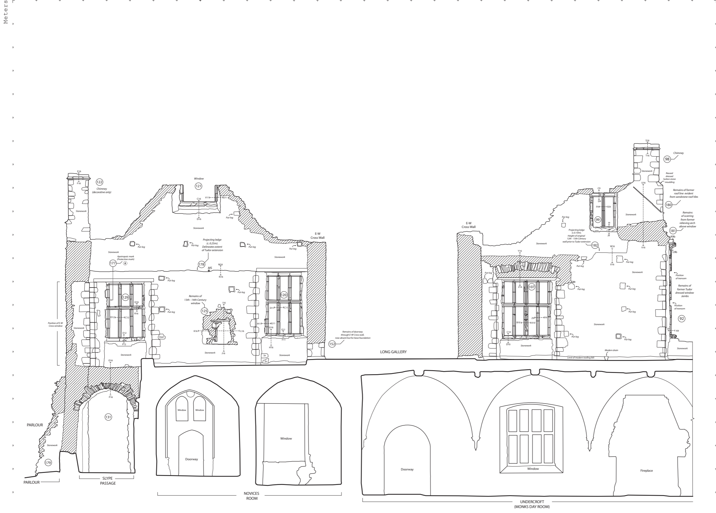
EAST WALL West Facing Elevation (Internal) - Northern end.
