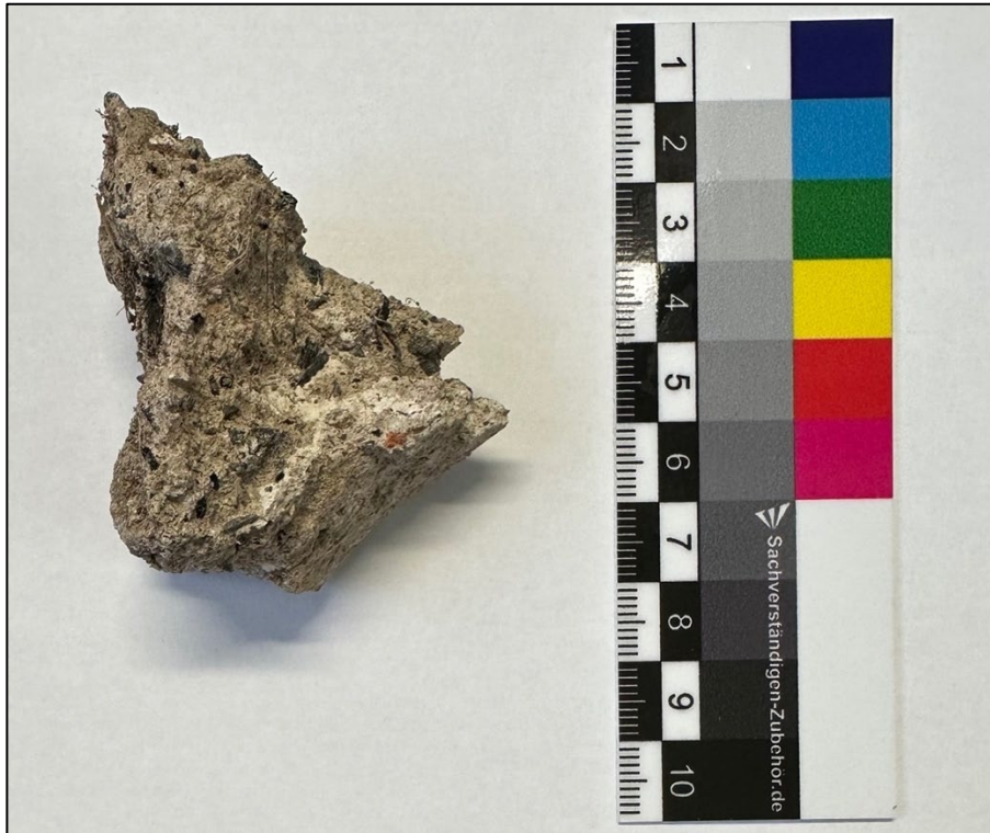
Plate 29. Location 13 NW Service Room, hard grey pozzolan ash (wood) mortar (*02) with stone aggregate inclusions overlying the west end of timber (w006), 18 th -19 th century.
