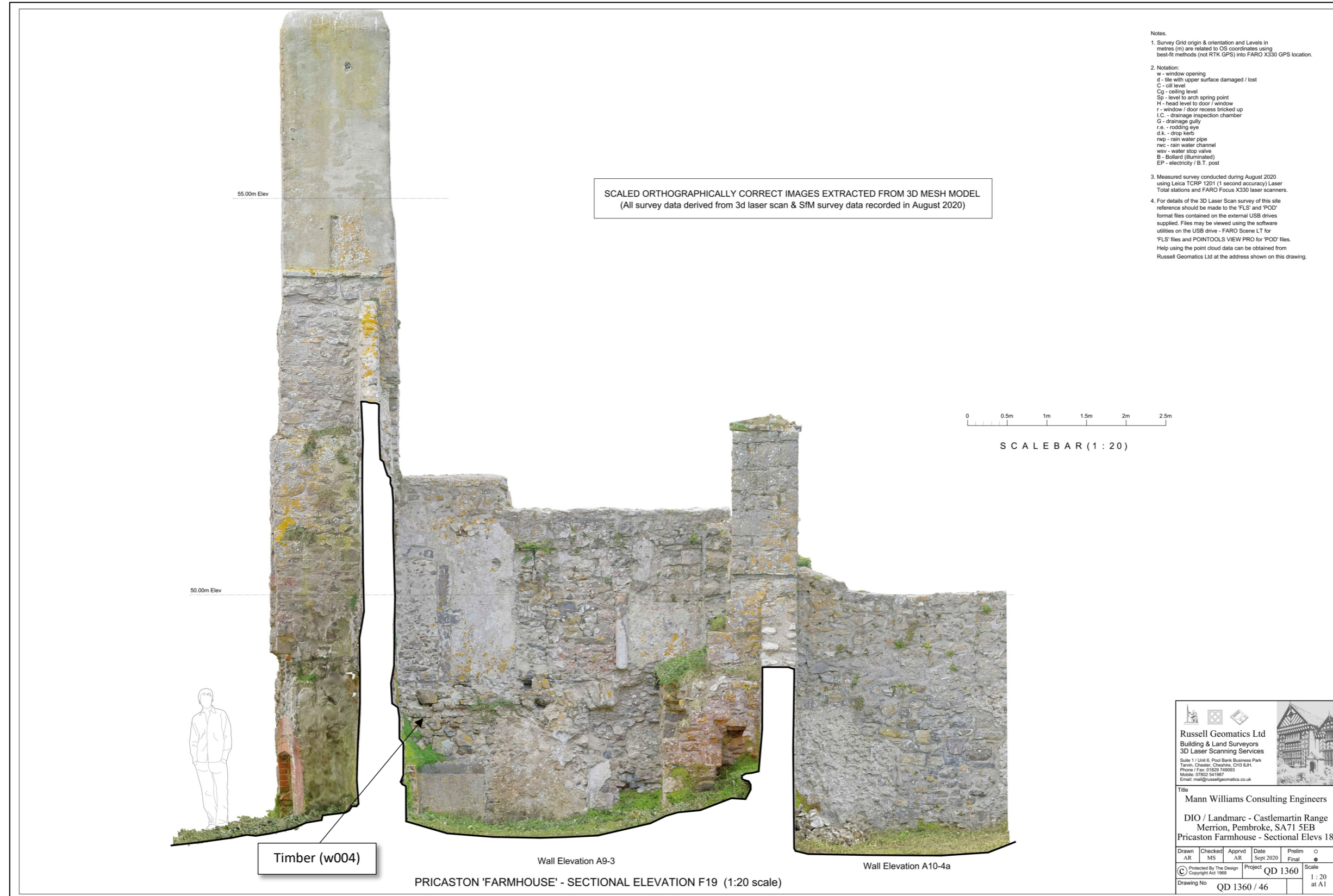
Figure 3. Laser and photogrammetric sections of Location 15, the medieval Tower ) before timber removal. (c) Russell Geomatics 2021.
