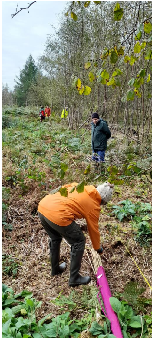
Fig. 6 Volunteers lay out the baseline. Transits were measured every 2m and marked at each end with bamboo canes. A yellow rope marked with highly visible marks every 0.5m was laid between the canes for each transit and data was collected manually, with the gradiometer 'pace' set to single shot at each mark. Photograph: Mark Lewis, 16-x-23 (written permissions to take and use photographs were signed by all participants and are archived by Buckholt Bryngaer CIC in accordance with GDPR).
