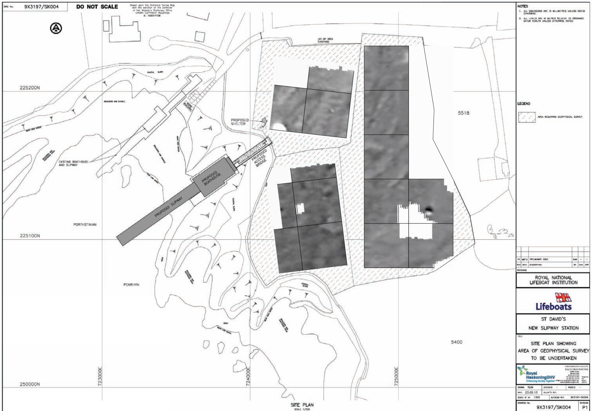
Fig 4: Geophysical survey results overlaid on site plan
