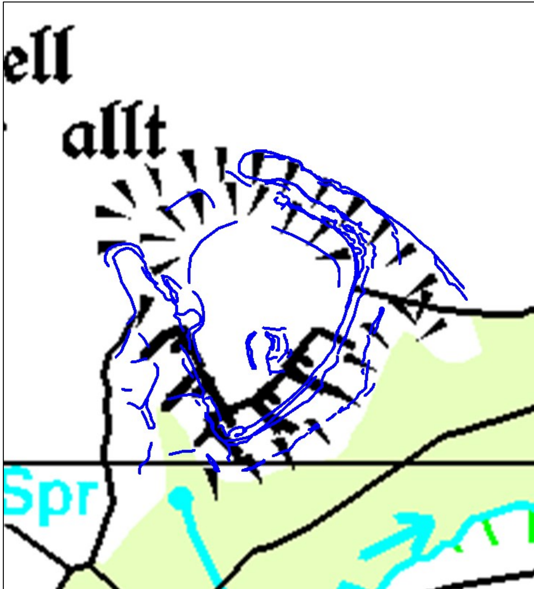
Figure 7: Topographical survey results for Castell Pen-yr-Allt, showing surveyed bank-tops in blue, with OS 1:10,000 backing map for comparison
